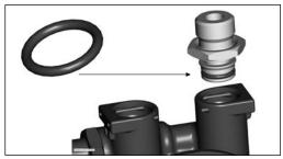
3 Insert the fittings, if provided, into the holes of the inlet and outlet of the pump to bring them beat on the body. While inserting the fittings do not use the motor as a pump support, in order to avoid a possible damage to itself. When inserting the fittings do not hold the pump with a wrench to prevent damage to itself.
